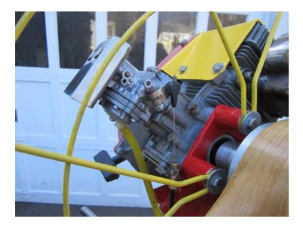
While making some of the pieces to hold the cable, that's when I came to a blinding flash that I didn't need a fuel tank as this carburetor has a fuel pump in it and could suck fuel just like the big boys! So all I needed was to bring fuel to the carburetor with fuel line, and a quick disconnect to connect to a remote gas tank. More pieces to make for the QD and add the fuel line to it and it's done.
