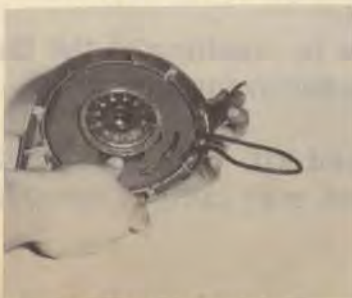
Elongated notch correctly positioned opposite cord outlet.
