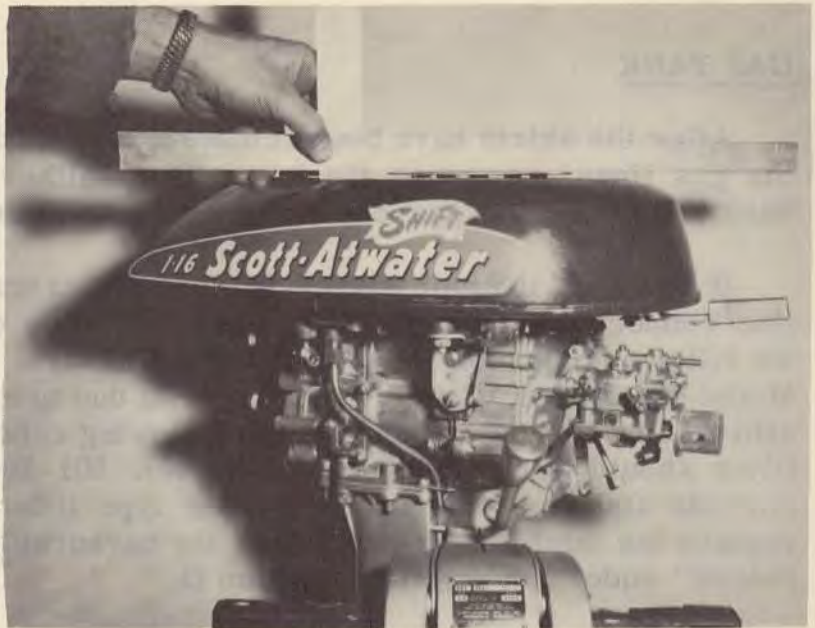
Measuring gas tank height.
