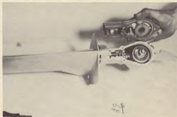
Testing for correct Reverse Lock Clearance on '50 models.
