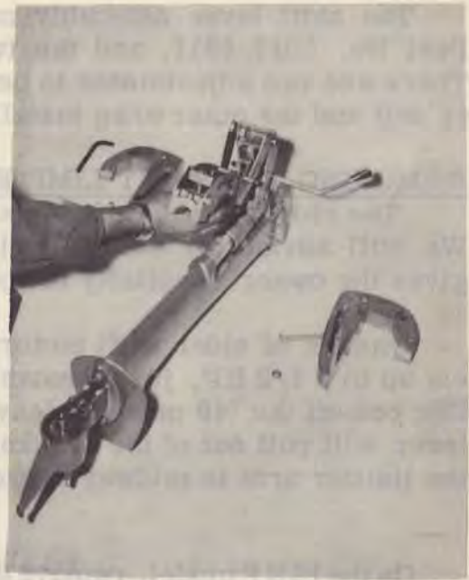
Replacing tilt arm assembly.
