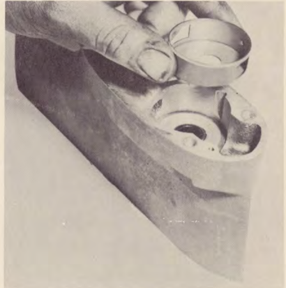
Dimple in the cup corresponding to the slot in the casting.
