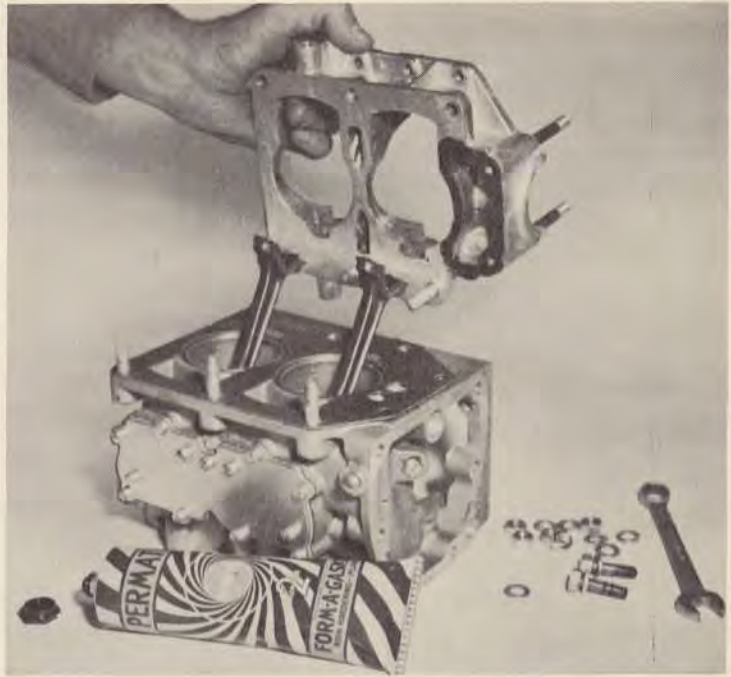
Replacing back half of crankcase.
