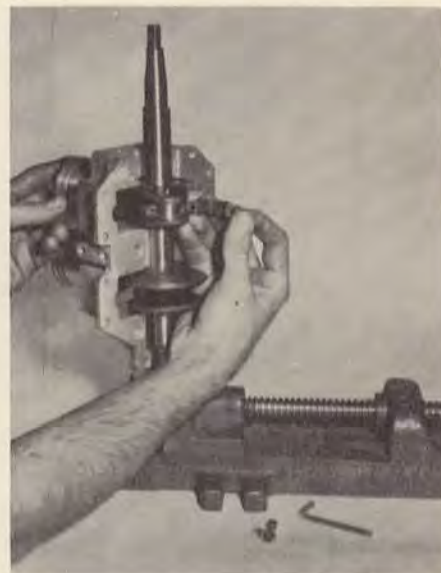
Installing rods on crankshaft.
