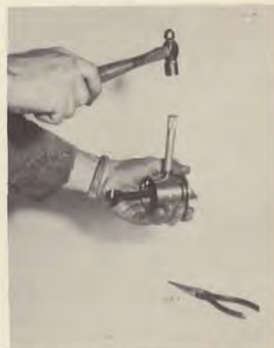
Attaching piston to rod.
