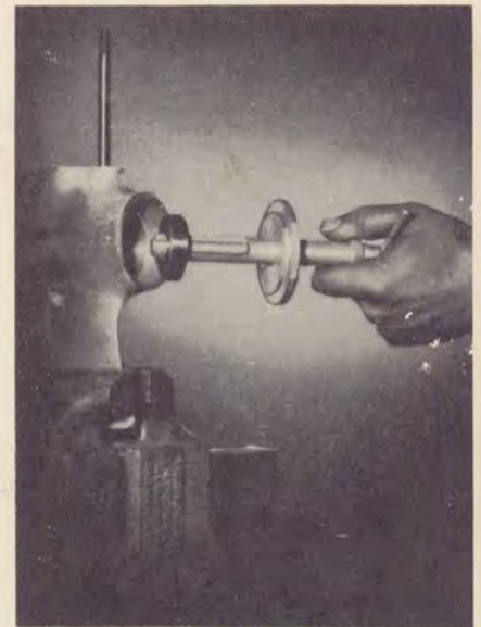
Removing front prop shaft bearing.
