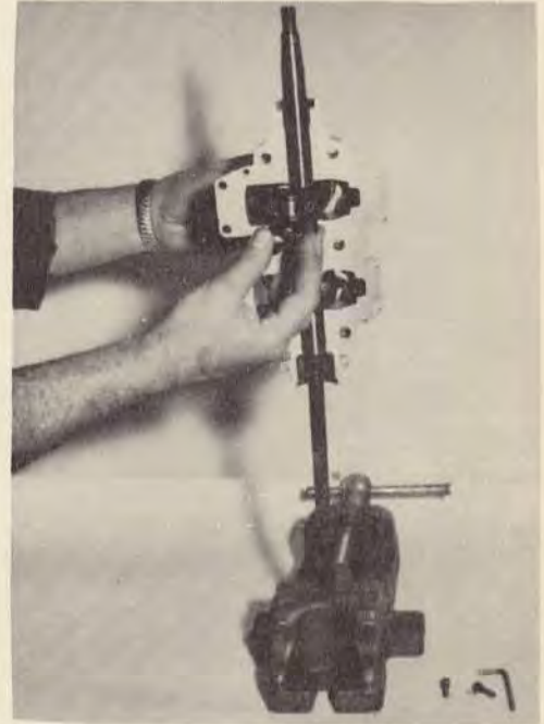
Attaching rods to crankshaft.
