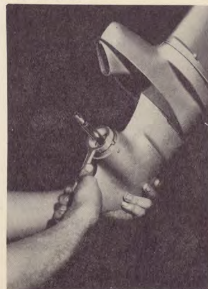
Removing lower unit cap. Tools shown in illustrations are A50-635 Lower Unit. Tool Set, $6.50 net per Set.
