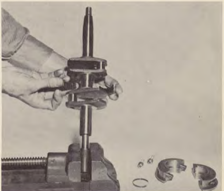
Installing Center main race.
