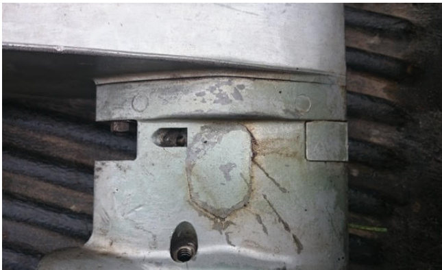
Standard Pusher Position (V block in FRONT)
