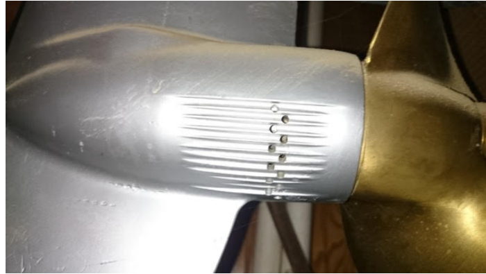
KF9 Water Intake Holes (above)
