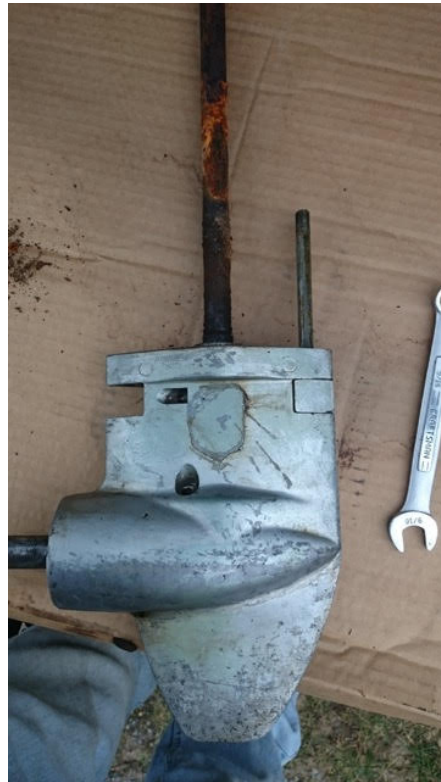
KF9 lower unit with V block installed on the leading edge for the standard "pusher" setup!
