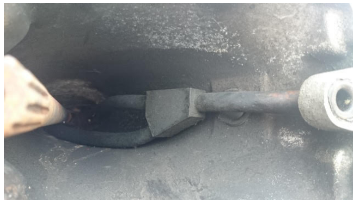
Looking down at the Y Pipe inside the lower unit!
