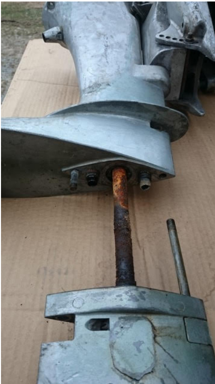
KF9 mid section and lower unit, partially disassembled to show where the Y pipe comes down from the powerhead!
