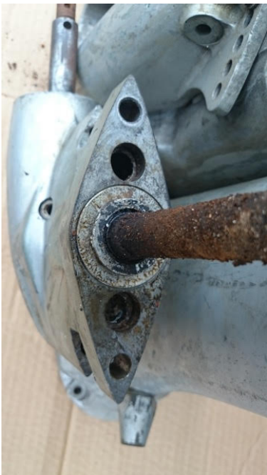
Looking down at the Y Pipe inside the lower unit!
