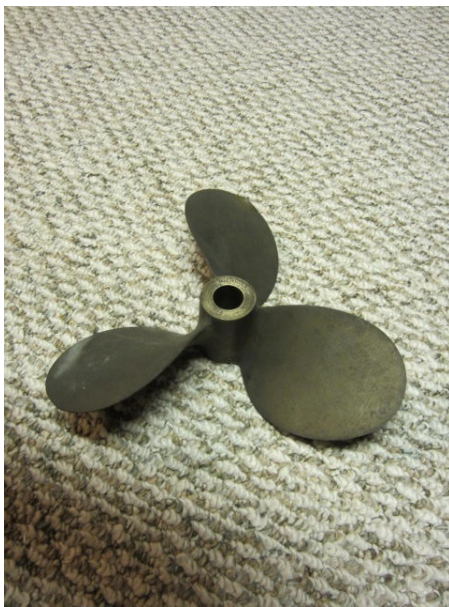
A right-hand rotation prop, that could have been used on the KF9 in Tractor Drive configuration.
