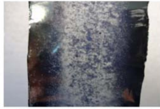
Plate failure due to corrosion.
