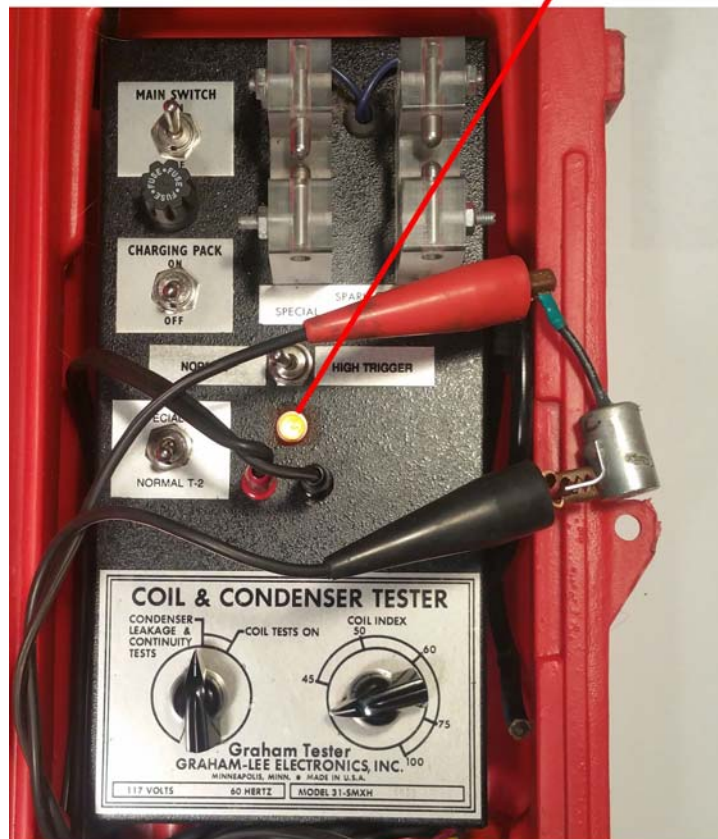
Fig. 4 - Using "Neon Lamp Style" Tester
