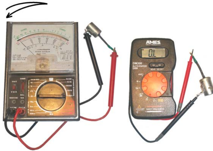
Fig. 1 - TESTING CONDENSER WITH OHMMETERS
