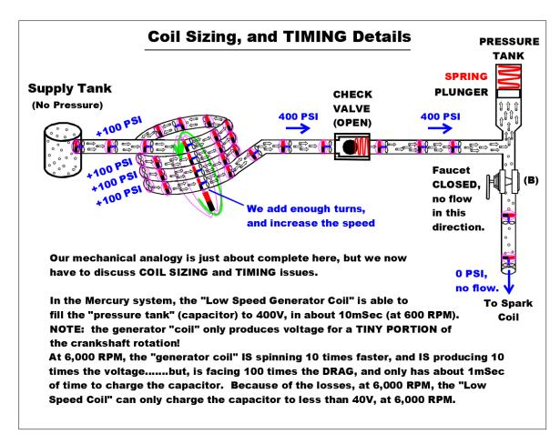
This is where everything comes together. For the "low speed generator coil", at LOW speeds, it's only producing about 400V, and is has enough TIME to be able to get most of that voltage into the capacitor.
