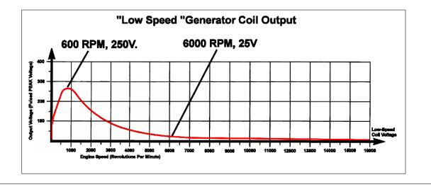
SO....the "low-speed generator coil" is GREAT for providing high voltage to our capacitor at very low speeds (even slightly under 100 RPM). It's output continues to rise up to 600 RPM, where the losses match the gains. At higher RPMs, the losses GREATLY OVEWHELM the voltage gains, and the output of this coil collapses. At above 2000 RPM, this coil is basically WORTHLESS, and above 4000 RPM, the engine would be misfiring.
