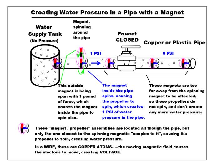
Magnets push electrons around in a wire....here we have magnets pushing water around in a pipe. Note that the faster you spin the magnet, the more water pressure you get......just like you get more voltage in a wire when a magnet spins by faster.
