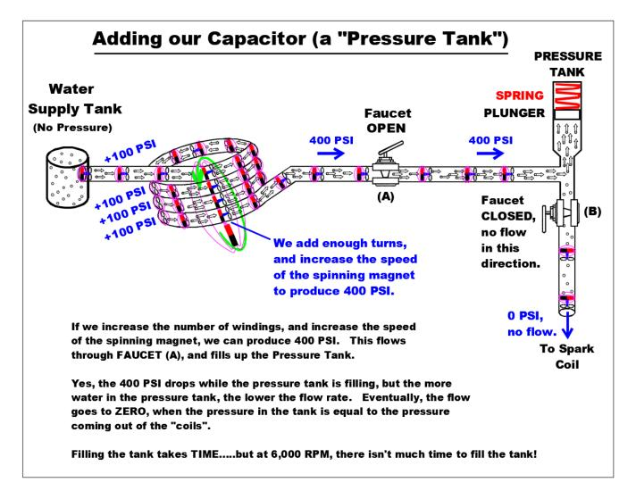
In the picture above, we have added our PRESSURE TANK (to simulate the capacitor in the Phase Maker ignition. And, we have added another pipe, that will allow the "capacitor" to empty out to our spark coil......when faucet "B" is closed.
