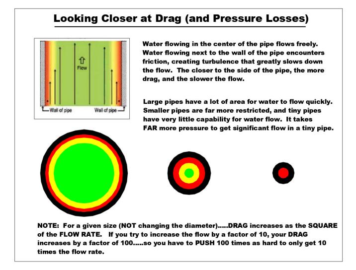
As this picture describes, DRAG increases as the SQUARE of the flow rate. To increase the flow by a factor of 10, you have to increase the PRESSURE by a factor of 100....(to overcome the increase in the drag.) This is a KEY CONCEPT, that Mercury took advantage of!
