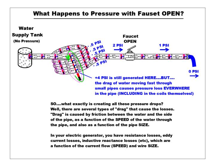
Here, we see that when water flows quickly, that "drag" causes pressure losses through the pipe. The longer the pipe, the more the losses. And, (a KEY CONCEPT here)....there's a LOT OF PIPE in that "coil". Before the faucet was opened, the COIL was producing 4 PSI (with NO LOSSES IN THE COIL.) But, if the water is flowing FAST, the DRAG inside the coil drops half of the pressure, even before it gets out of the coil. Further down the pipe, the "drag" created addition losses.
