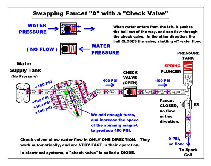
The picture above shows how "check valves" work. I think we all are familiar with these, right? Well, ELECTRICAL terms, these are known as DIODES. (In the Phase Maker schematic, I show where these are located in that early CDI ignition system).
