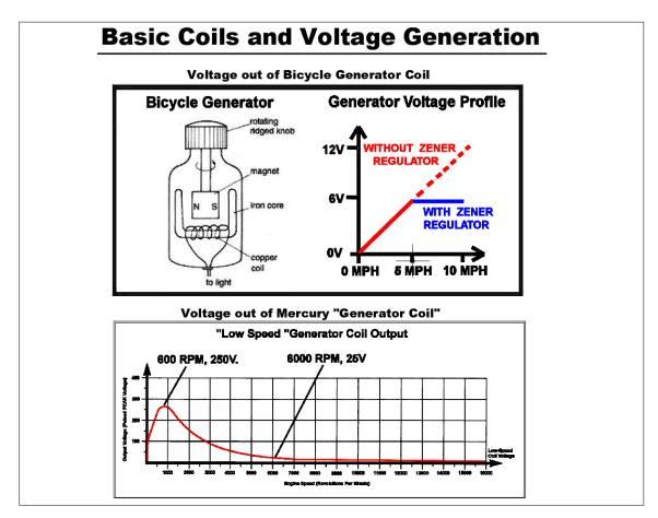
Then, along comes Mercury, claiming that the coils in their generators rise up to a peak at a specified RPM, then automatically limit (then reduce) their output voltage, without any external circuitry whatsoever. (See the lower diagram, above)
