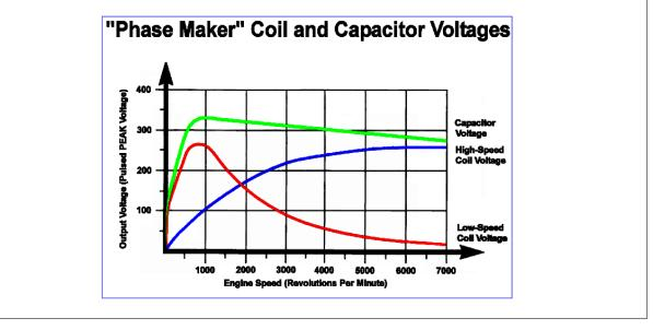
A KEY POINT TO REMEMBER is that in CDI ignition systems, the capacitor only gets the charge from ONE PULSE of the flywheel magnets moving past the generator coils. The capacitor is then COMPLETELY DISCHARGED through the spark coil....and the cycle repeats over and over and over.
